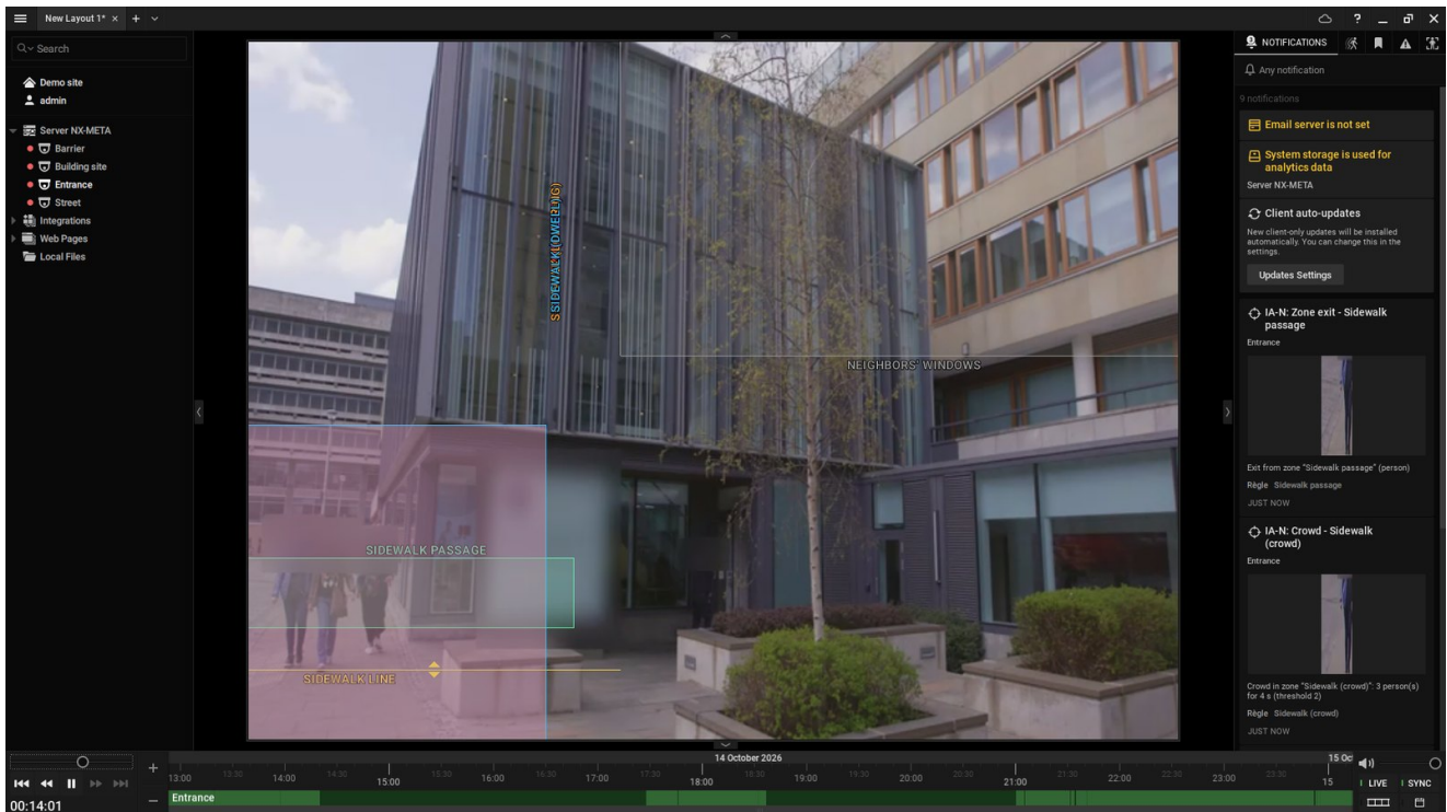
Screenshot 1 — Live IA-N alarms: VMS notifications in the right panel (type, zone, camera, thumbnail, alarm text).
