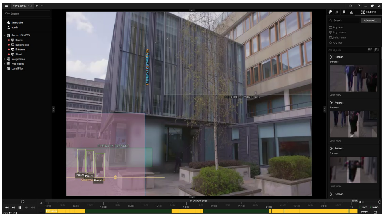
Screenshot 4 — “Objects” tab: boxes on the image and list of the objects detected by IA-N Analyse, with the filters.
