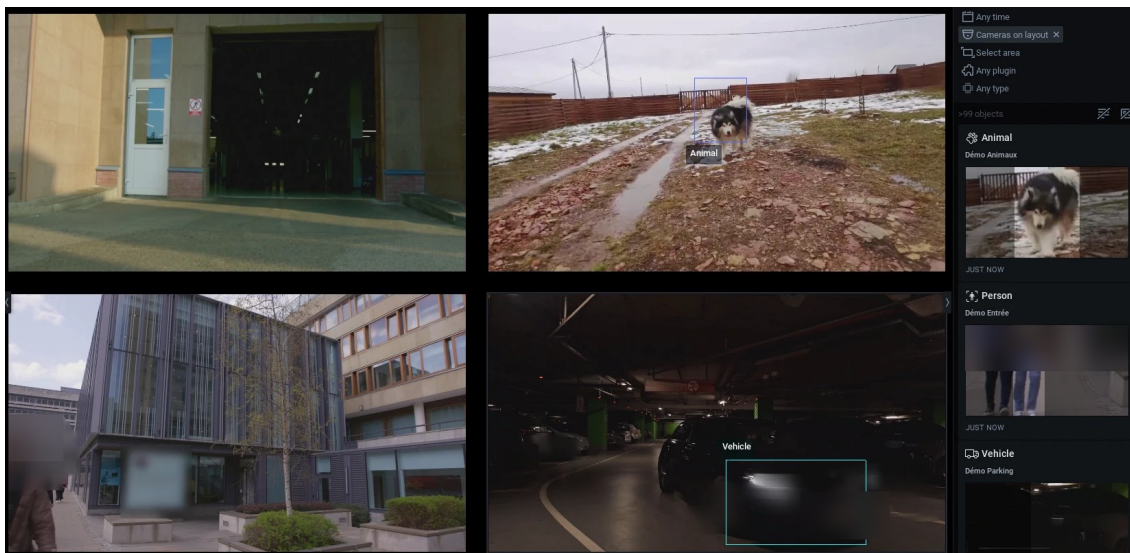
Real capture of the VMS client (client in English): "Animal" and "Vehicle" boxes, object list on the right with the "Any plugin" and "Any type" filters. Faces and plates blurred.
