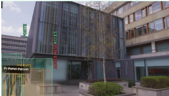
1 · In the VMS client: zones "Porte" and "Accès" (real capture)
